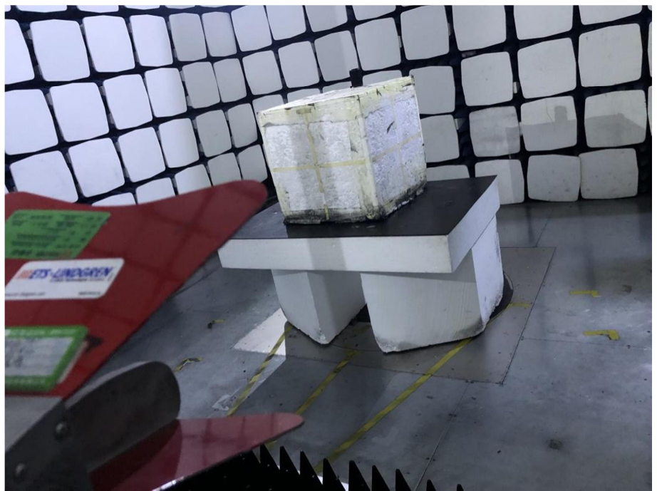
Radiation Emission Test Setup (1GHz to 18GHz)
