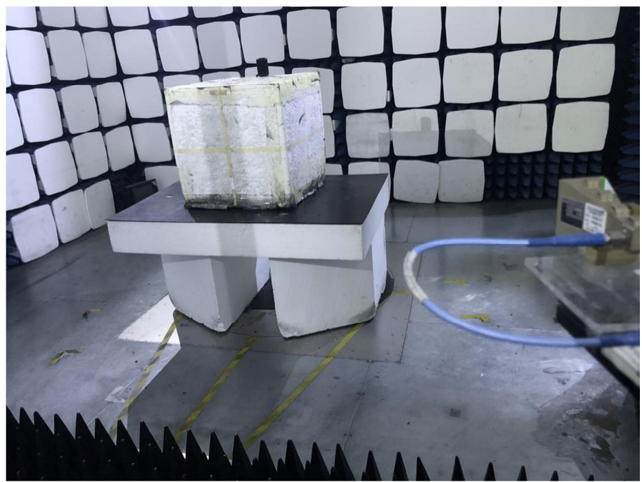
Radiation Emission Test Setup (Above 18GHz)
