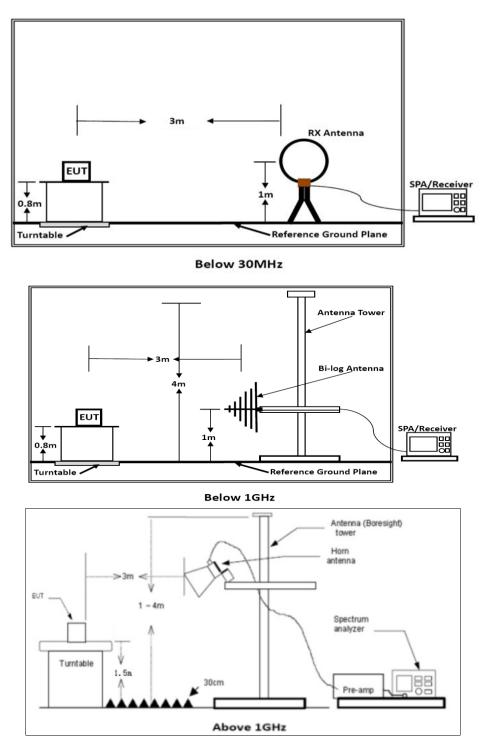
Above 18 GHz shall be extrapolated to the specified distance using an extrapolation factor of 20 dB/decade form 3m to 1m.
