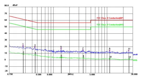
AC Conducted Emission of GFSK high channel @ AC 120V/60Hz @ GFSK (worst case) Line
