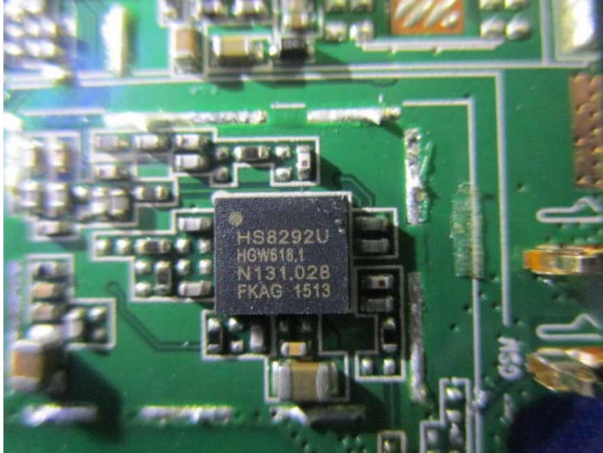
EUT –GSM Transceiver Chip View
