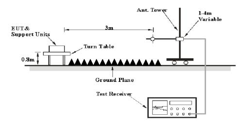
The radiated emission tests were performed in the 3 meters chamber test site for the range 30MHz to 1GHz and the 3 meters chamber test site for above 1GHz, using the setup accordance with the ANSI C63.4-2014. The specification used was the FCC Part 15.109 Class B limits.
