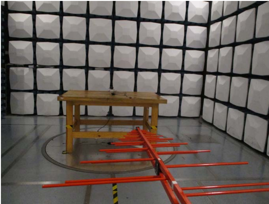
Radiated Emission View (Below 1GHz)
