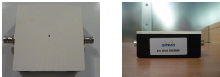
Figure 1 – Satimo COMOHAC Magnetic Field Simulator
