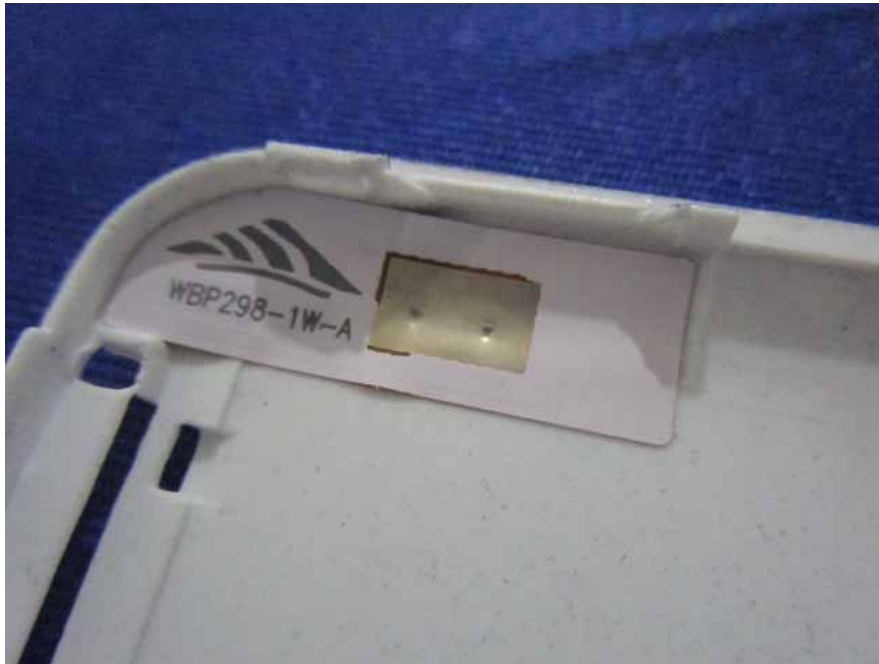
EUT -Wifi &BT Antenna View
