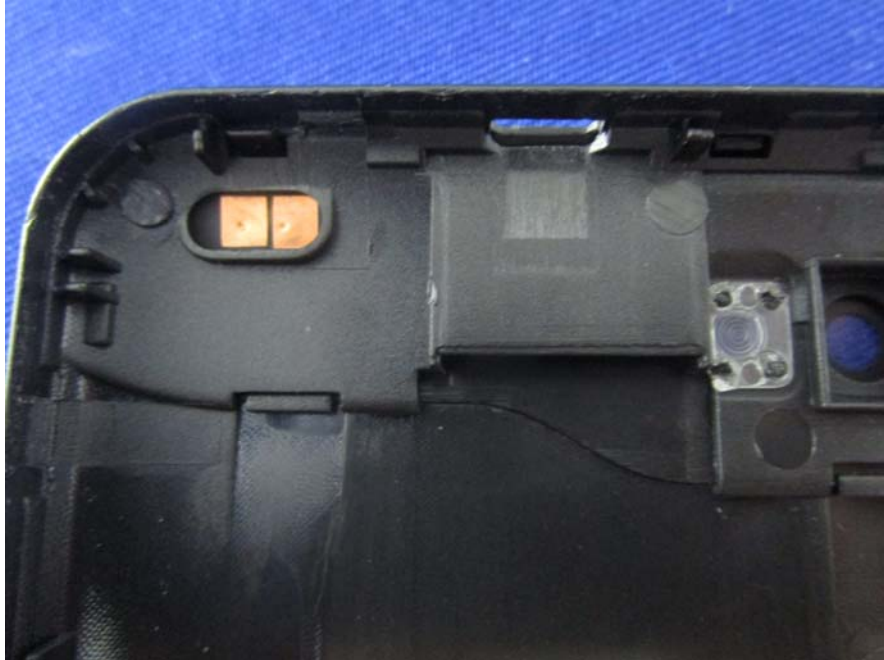
EUT – LTE RX Antenna View
