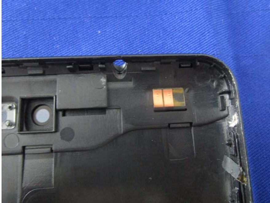
EUT – Wifi& BT Antenna View
