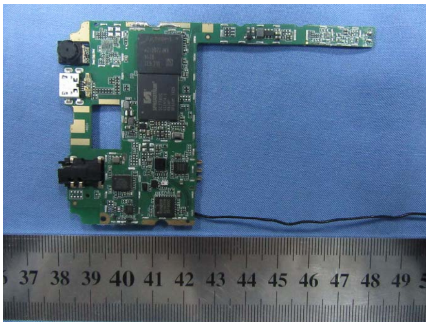
EUT – Main Board Uncover View
