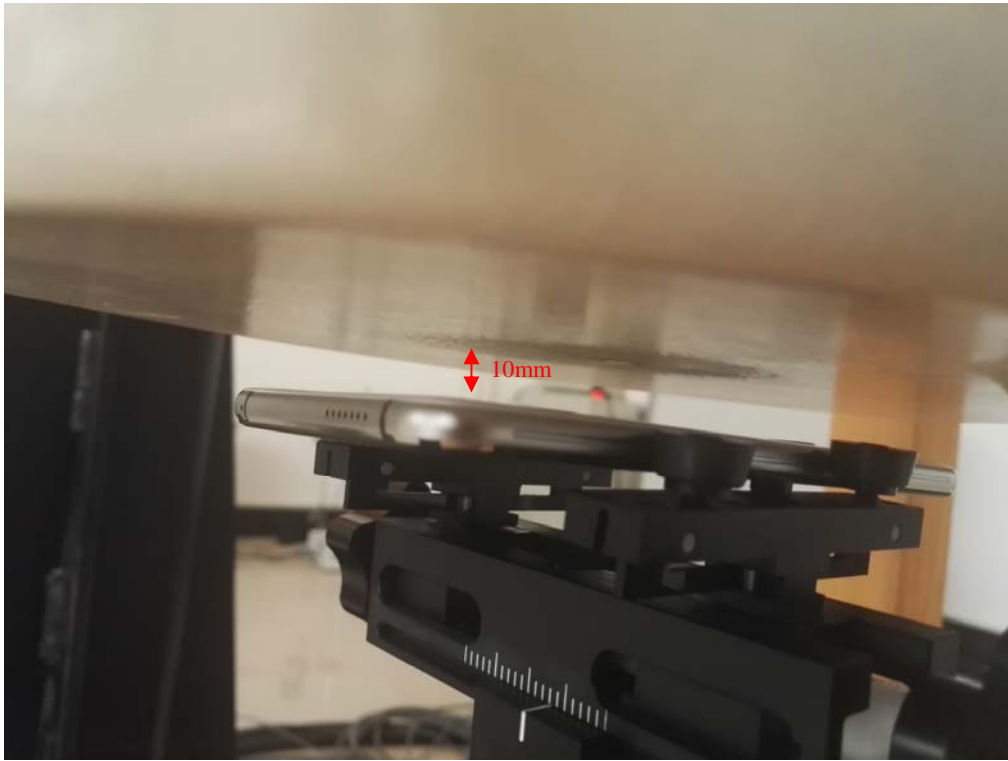
Body-worn Back Setup Photo (10mm)
