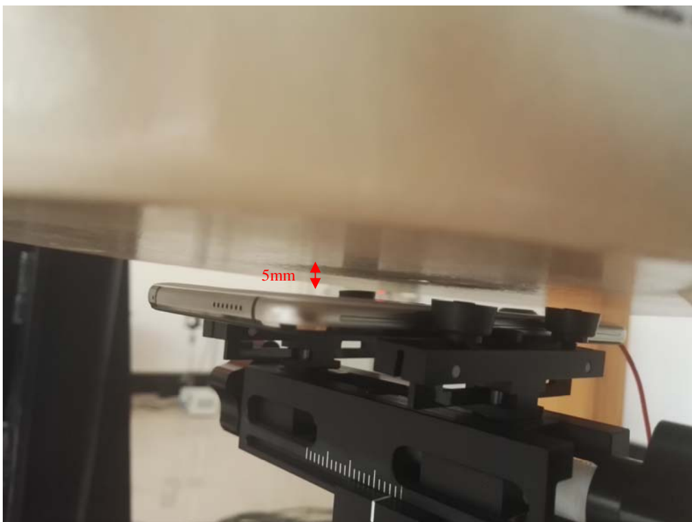
Body-worn- Back Setup Photo (5mm)
