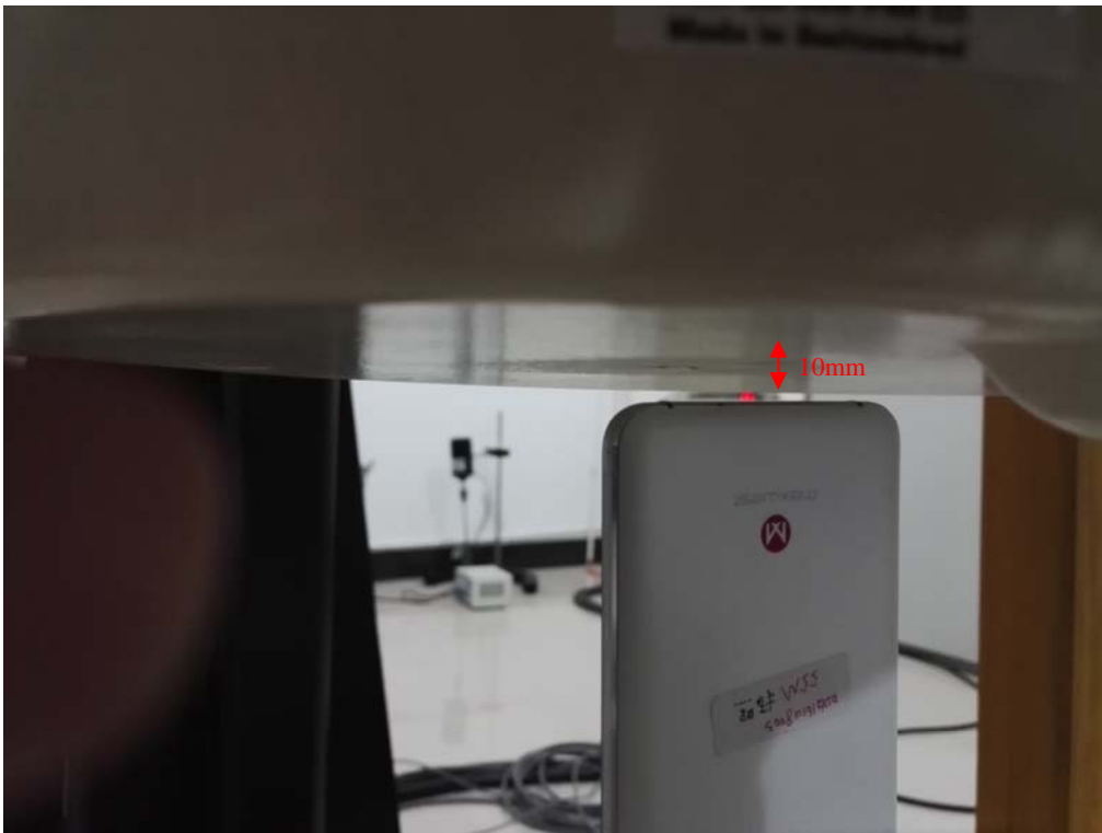
Body-worn Bottom Setup Photo (10mm)
