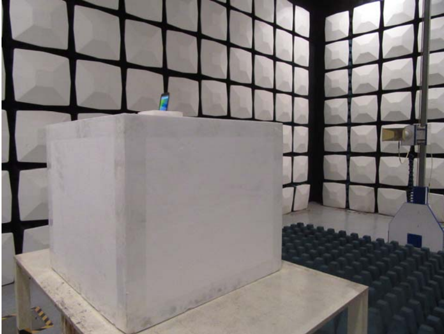
Radiated Emission View (Above 1GHz)
