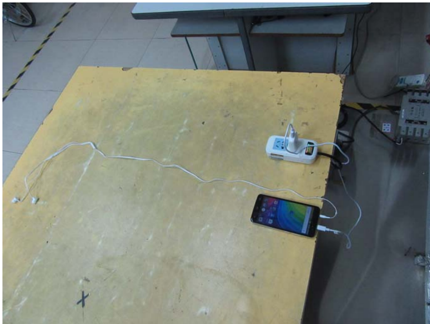
Conducted Emissions – Side View
