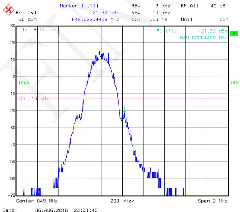
**GSM 1900, Left Band Edge**
