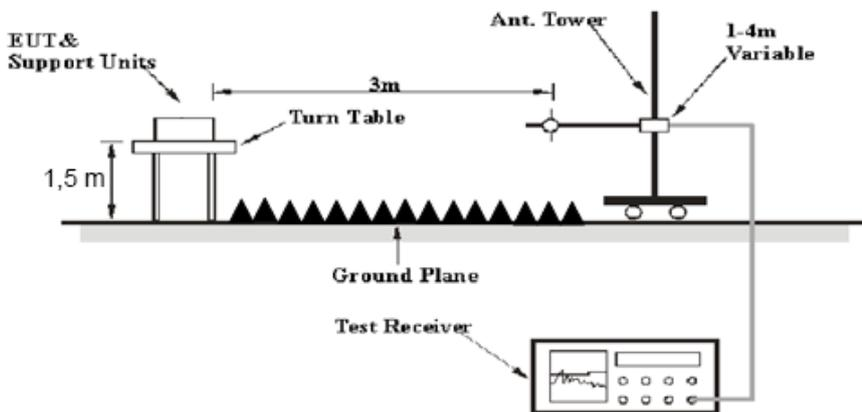
The radiated emission below 1GHz tests were performed in the 10 meters chamber, above 1GHz tests were performed in the 3 meters chamber test site B, using the setup accordance with the ANSI C63.10-2013. The specification used was the FCC 15.209, and FCC 15.247 limits.
