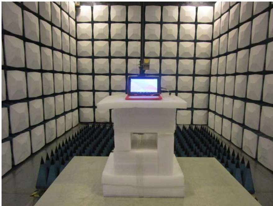
Radiated Emission View (Above 1GHz)
