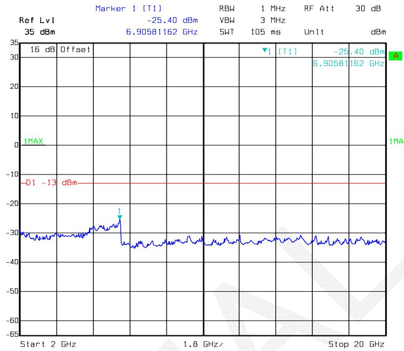
**QPSK, Band 2-10M \_ Middle Channel**
