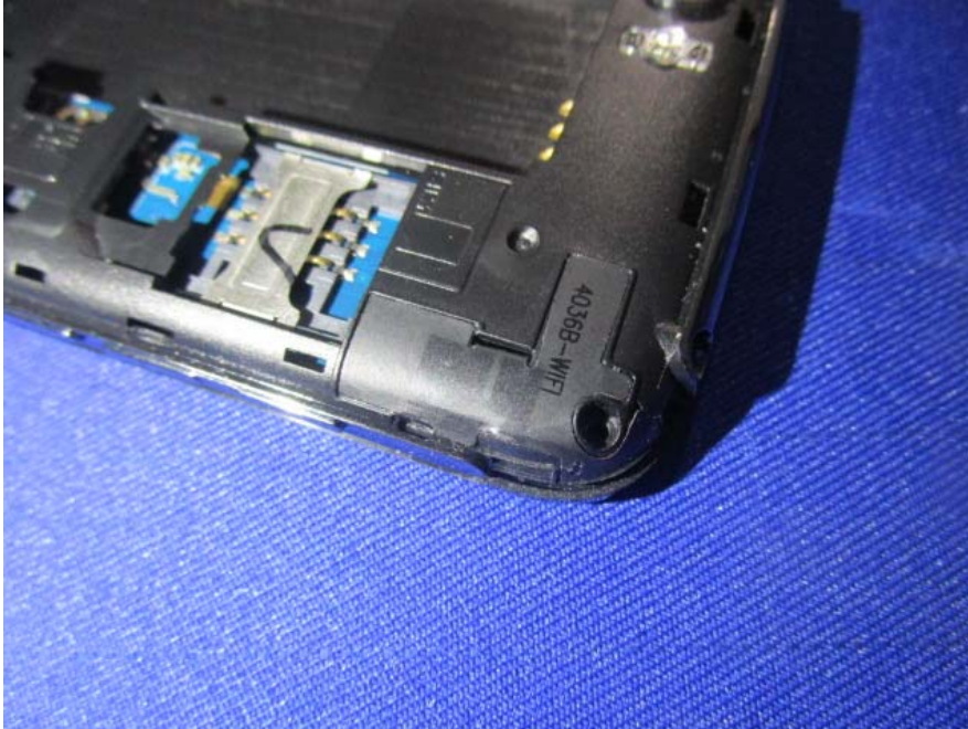
EUT -WiFi & BT Antenna View
