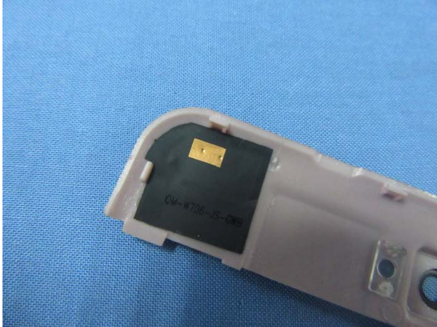
EUT – Wifi& BT Antenna View
