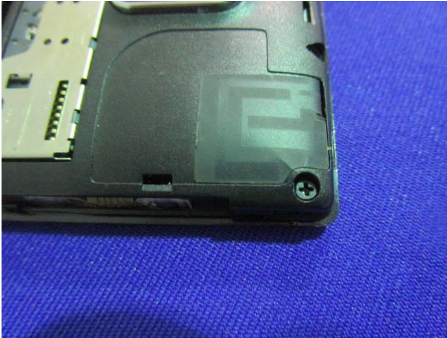
EUT –Wifi & BT Antenna View
