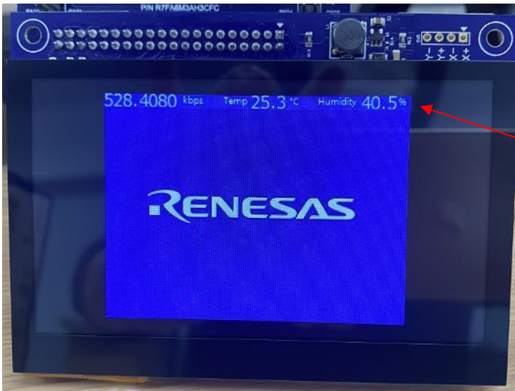
Display of throughput, temperature and humidity
