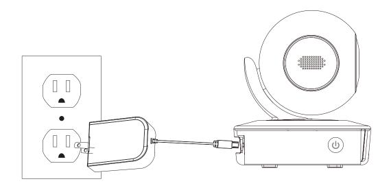
2.turn on the device, the camera system will self checking untill announce "ready for connection"
