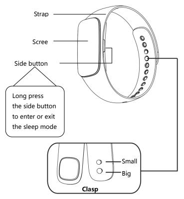
Please make sure the clasp is installed correctly
