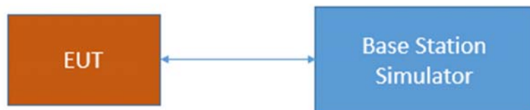
Test Setup FCC Part 22/24/27/90 Cellular; Frequency stability
