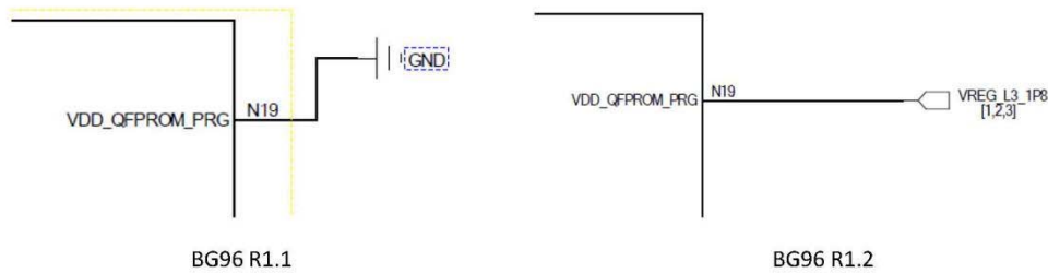
Figure 1: Schematic Designs of BG96 R1.1 and R1.2
