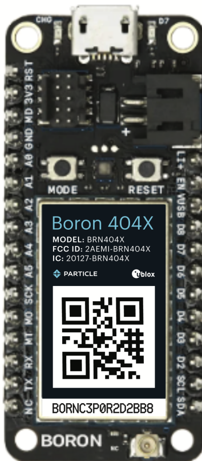
Label Location - Affixed to RF shield cover of EUT, top side Material: High temperature label
