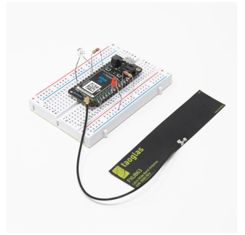
The Particle Boron is a mesh and Bluetooth development kit designed for building connected projects and products. To set up the device you'll need an Android or iOS mobile phone and a connection to the internet.
