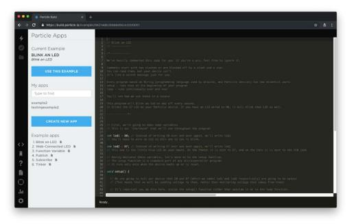
The code is heavily commented to help you understand the general structure of the sketch: the first part of the code declares two variables, the setup() function configures two pins as outputs, and finally the loop() which turns the onboard LED on, then off, then loops continuously.
