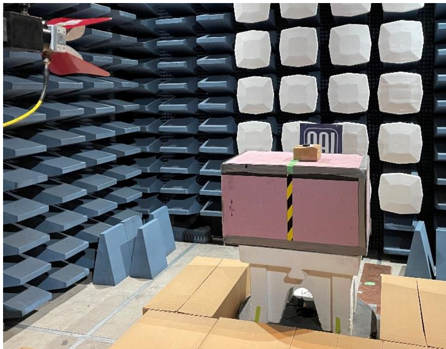
Figure 1: Intentional radiated emissions 1GHz – 18GHz
