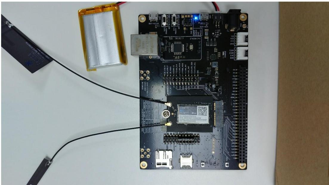
The Particle B402 is a mesh and Bluetooth development kit designed for building connected projects and products. To set up the device you'll need an Android or iOS mobile phone and a connection to the internet.
