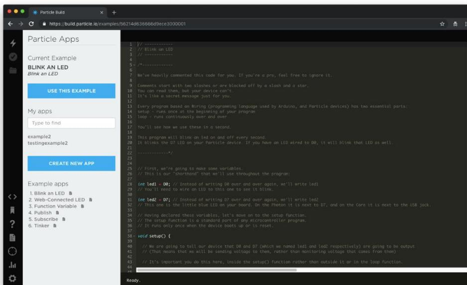
The code is heavily commented to help you understand the general structure of the sketch: the first part of the code declares two variables, the setup() function configures two pins as outputs, and finally the loop() which turns the onboard LED on, then off, then loops continuously.
