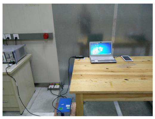
FCC RADIATED EMISSION TEST SETUP
