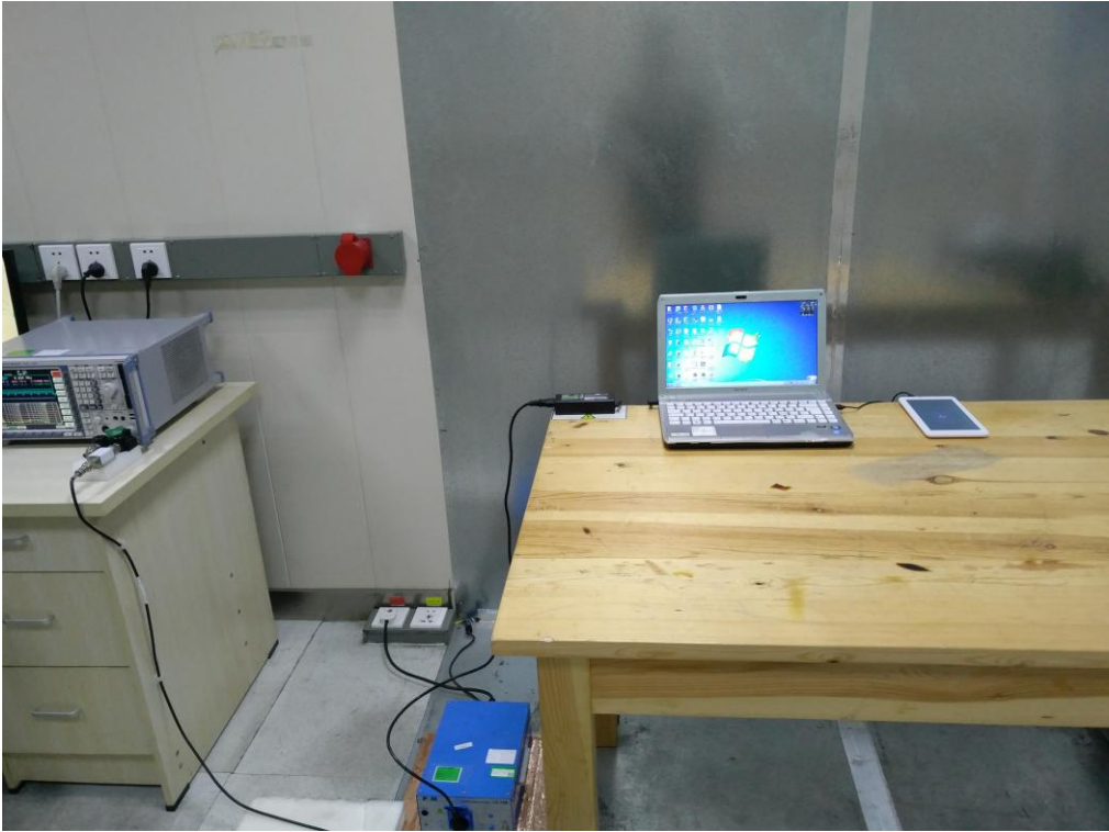
FCC RADIATED EMISSION TEST SETUP
