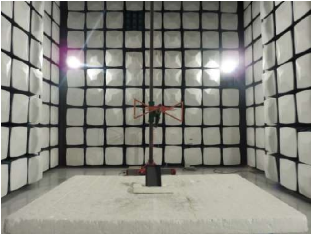
FCC RADIATED EMISSION TEST SETUP
