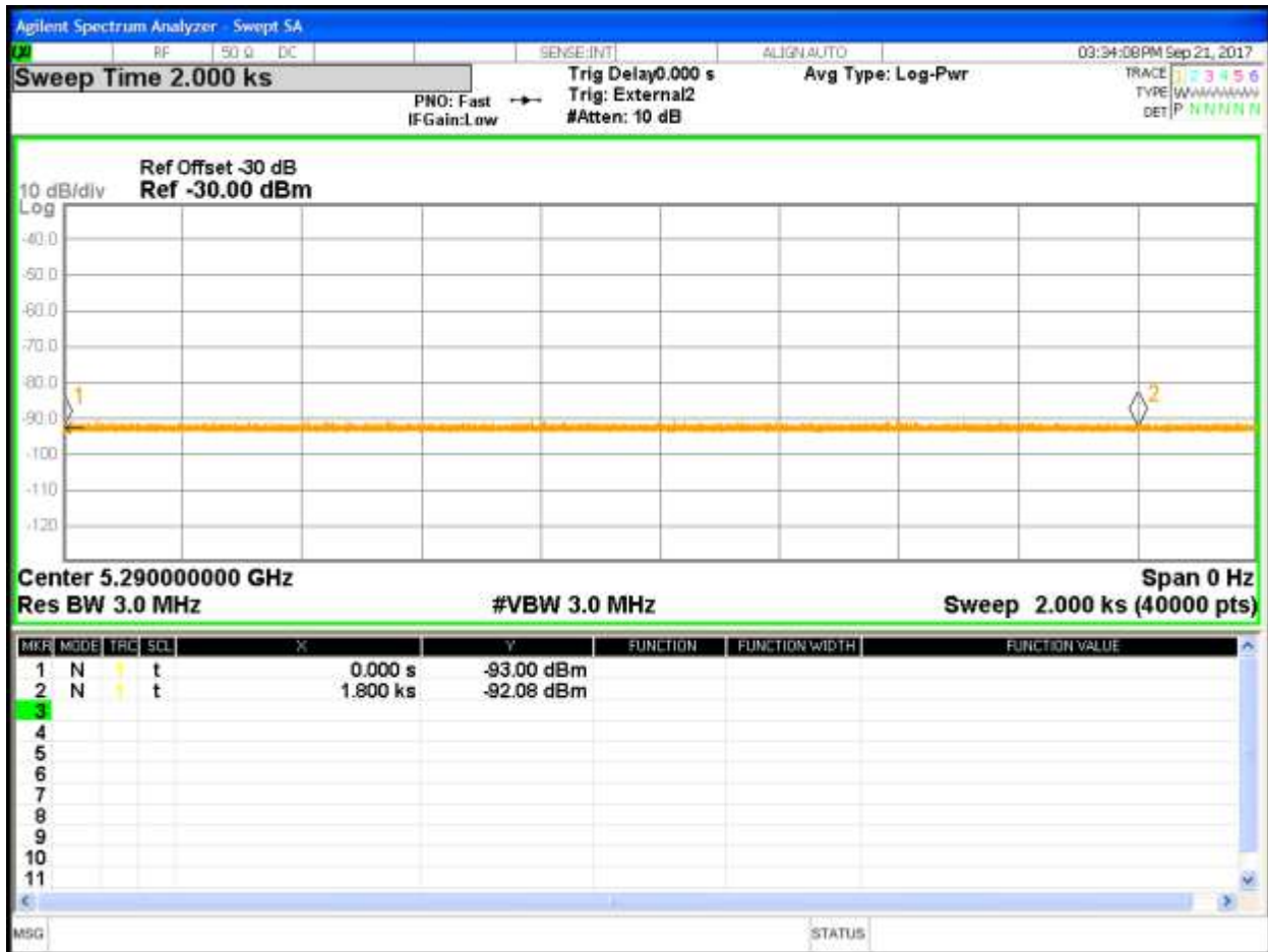
Figure 36: Non-Occupancy Period using Waveform Type 0 in Master Mode for 11AC VHT80, 80 MHz Bandwidth
