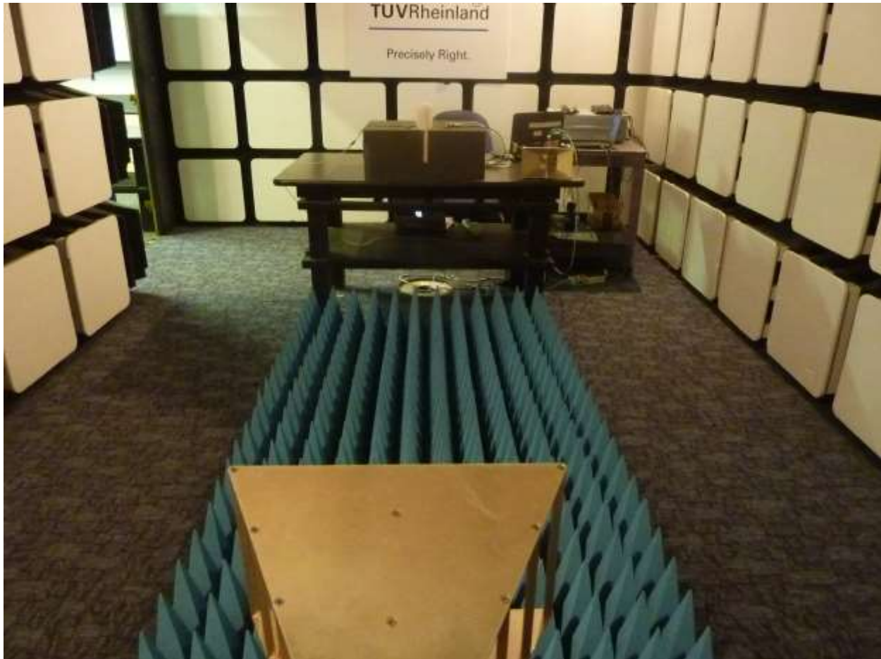
Figure 38: DFS Test Setup Photo for Master
