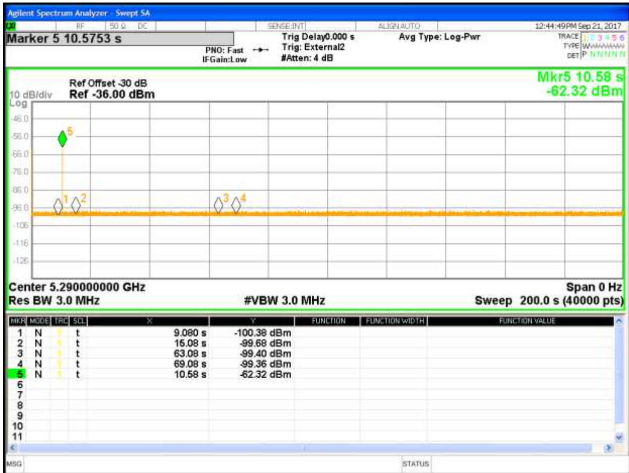
Figure 32: Radar Pulse Injection near the Beginning of Channel Availability Check for 80 MHz Bandwidth
