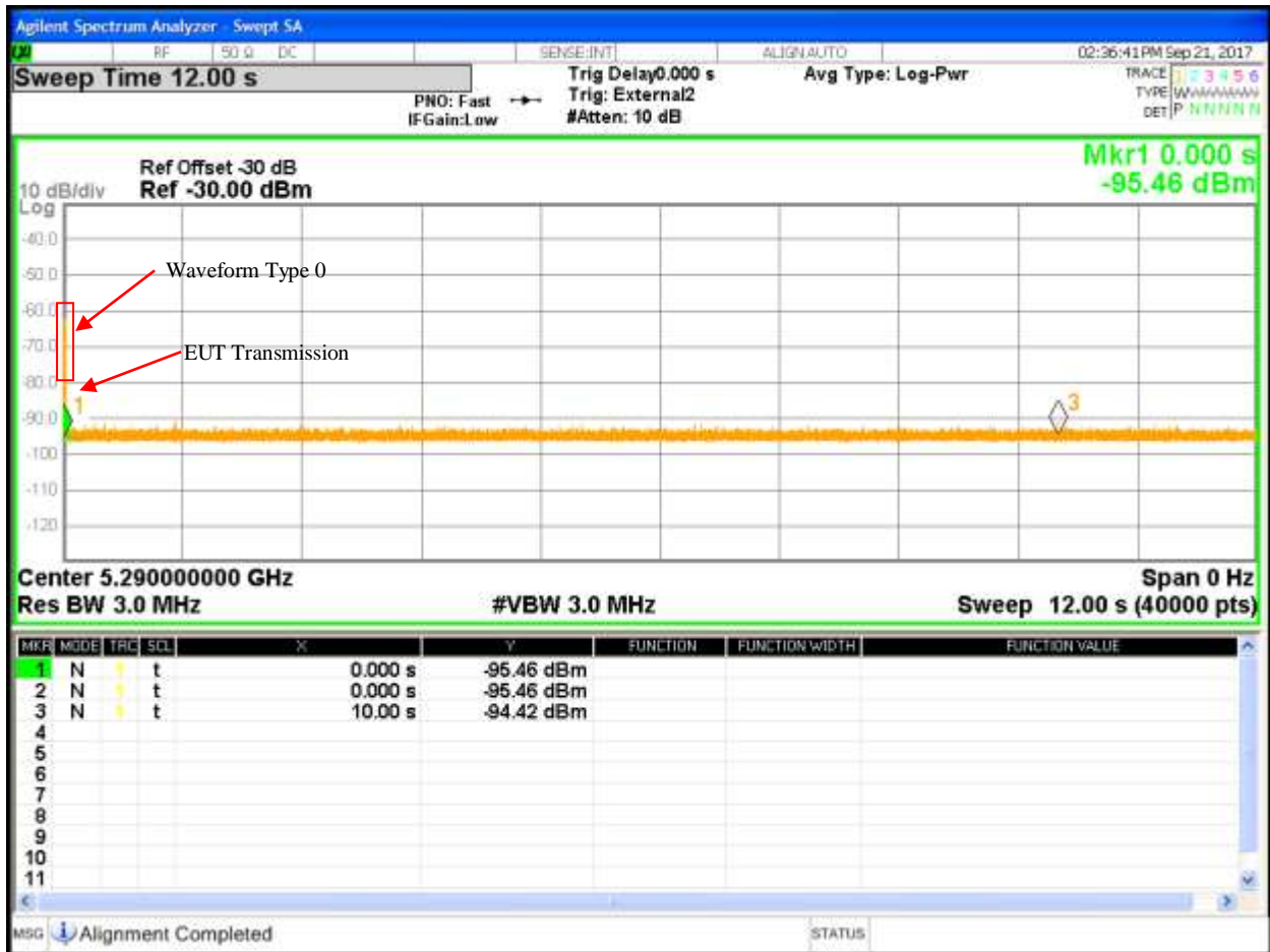
Figure 34: Channel Move Time and Channel Closing Transmission Time using Pulse Radar Waveform 0 in Master Mode 11AC VHT80, 80 MHz Bandwidth
