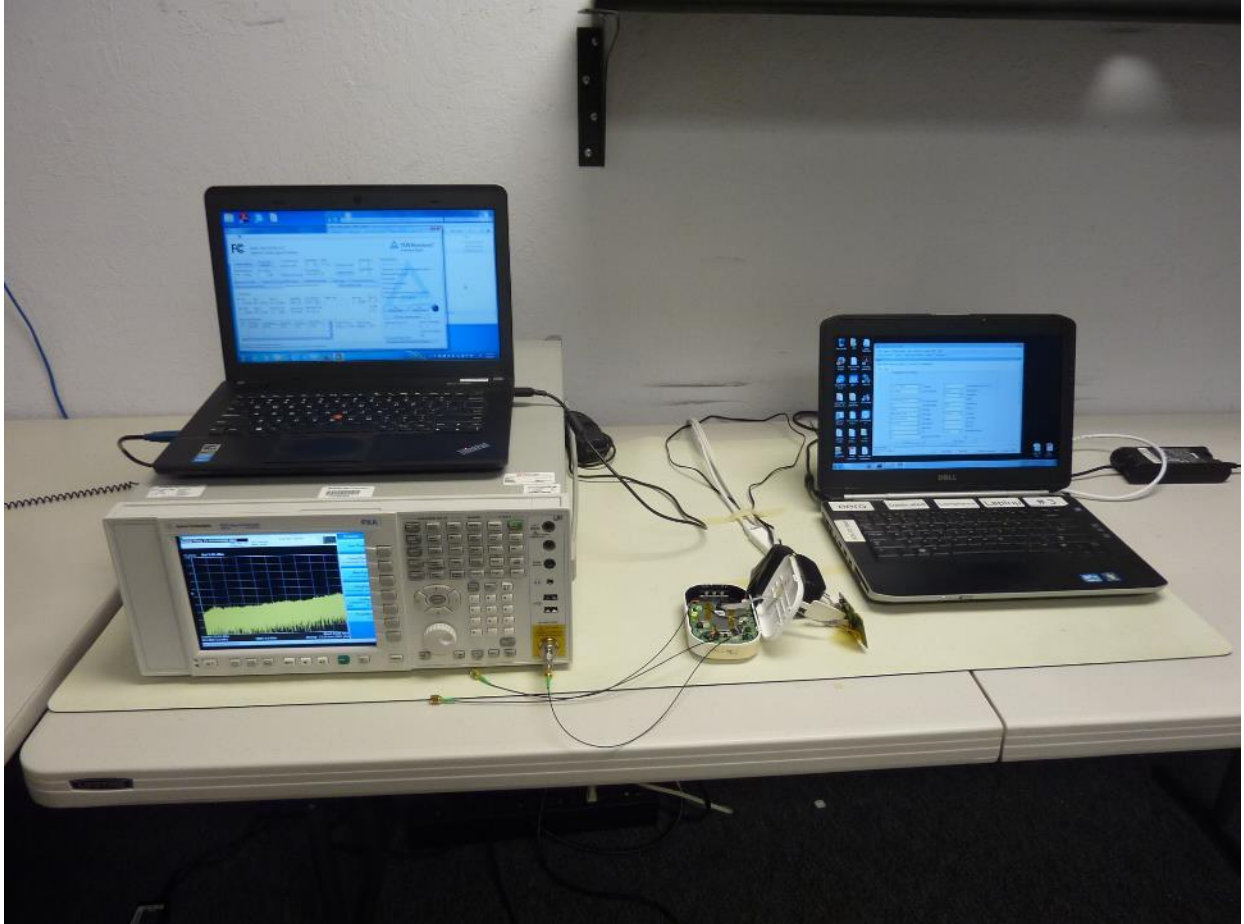
Figure 7: RF Conducted Test Setup
