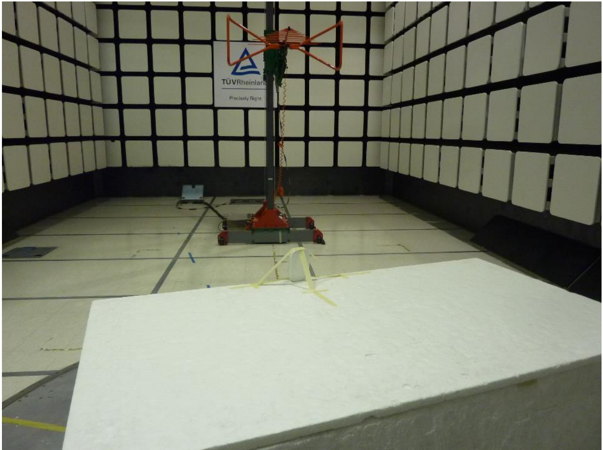
Figure 1: Test Setup for 30 MHz to 1000MHz (Front View)
