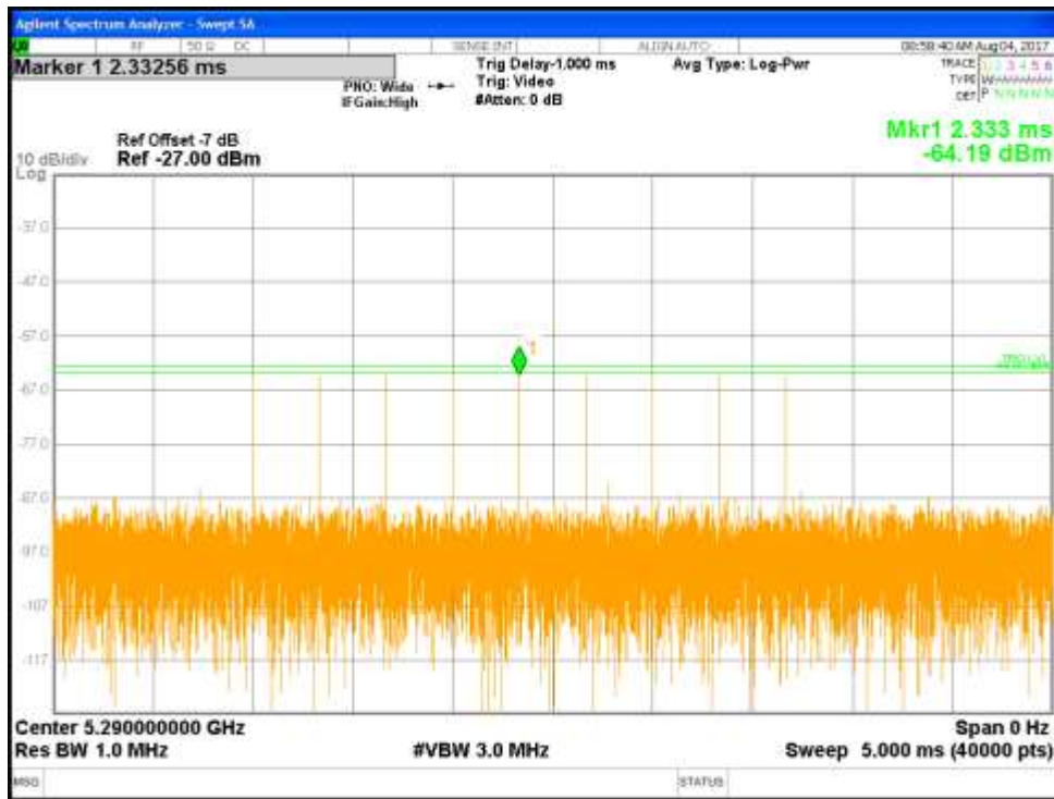
Figure 24: Radar Type 6 DFS Detection Threshold Level at 5290 MHz (9 Pulses in Burst)
