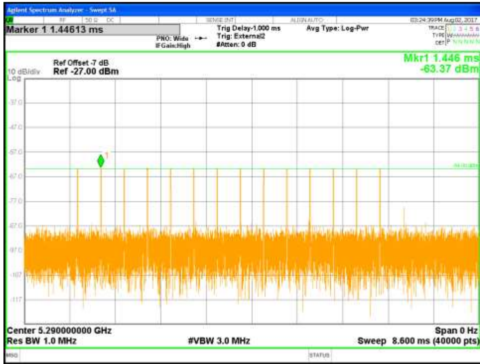
Figure 18: Radar Type 4 DFS Detection Threshold Level at 5290 MHz
