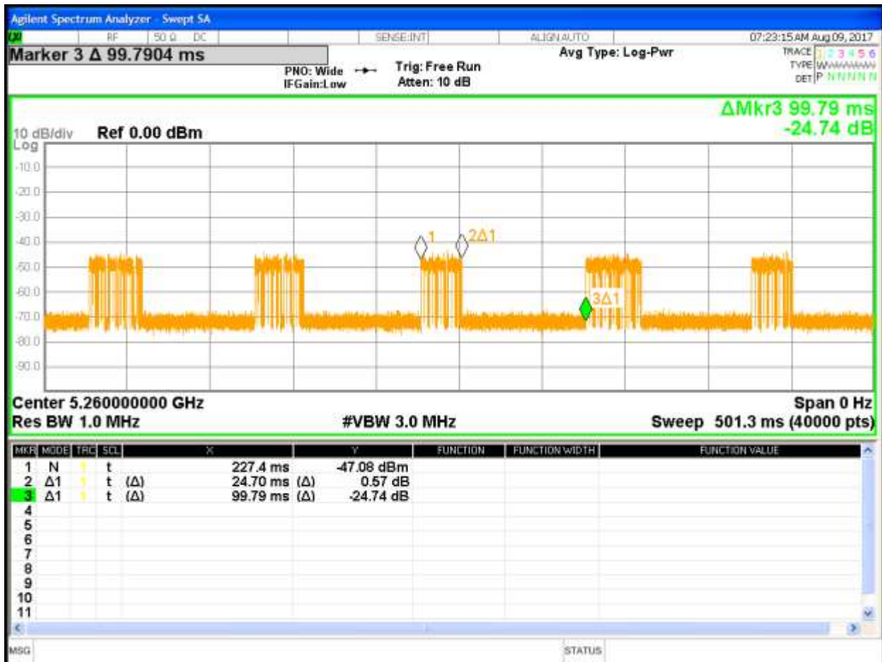
Figure 25: EUT Channel Loading at 5260 MHz (20 MHz bandwidth)
