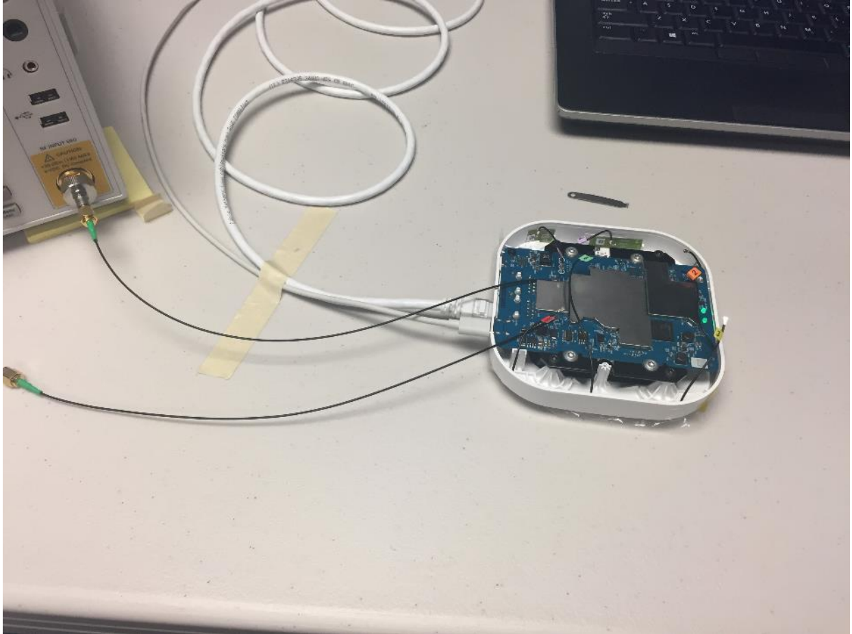
Figure 7: RF Conducted Test Setup – Closeup
