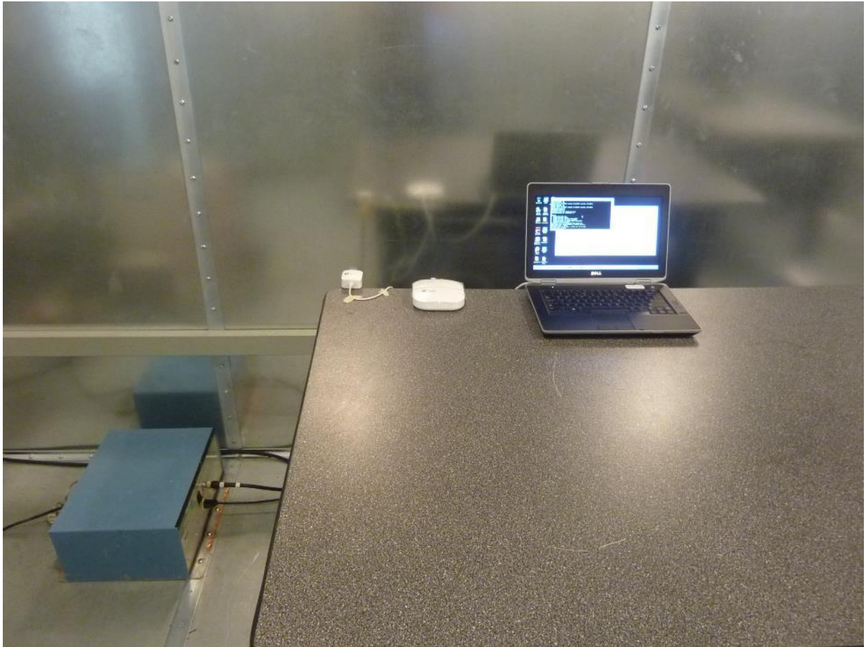
Figure 8: Conducted Emission Test Setup (Front)
