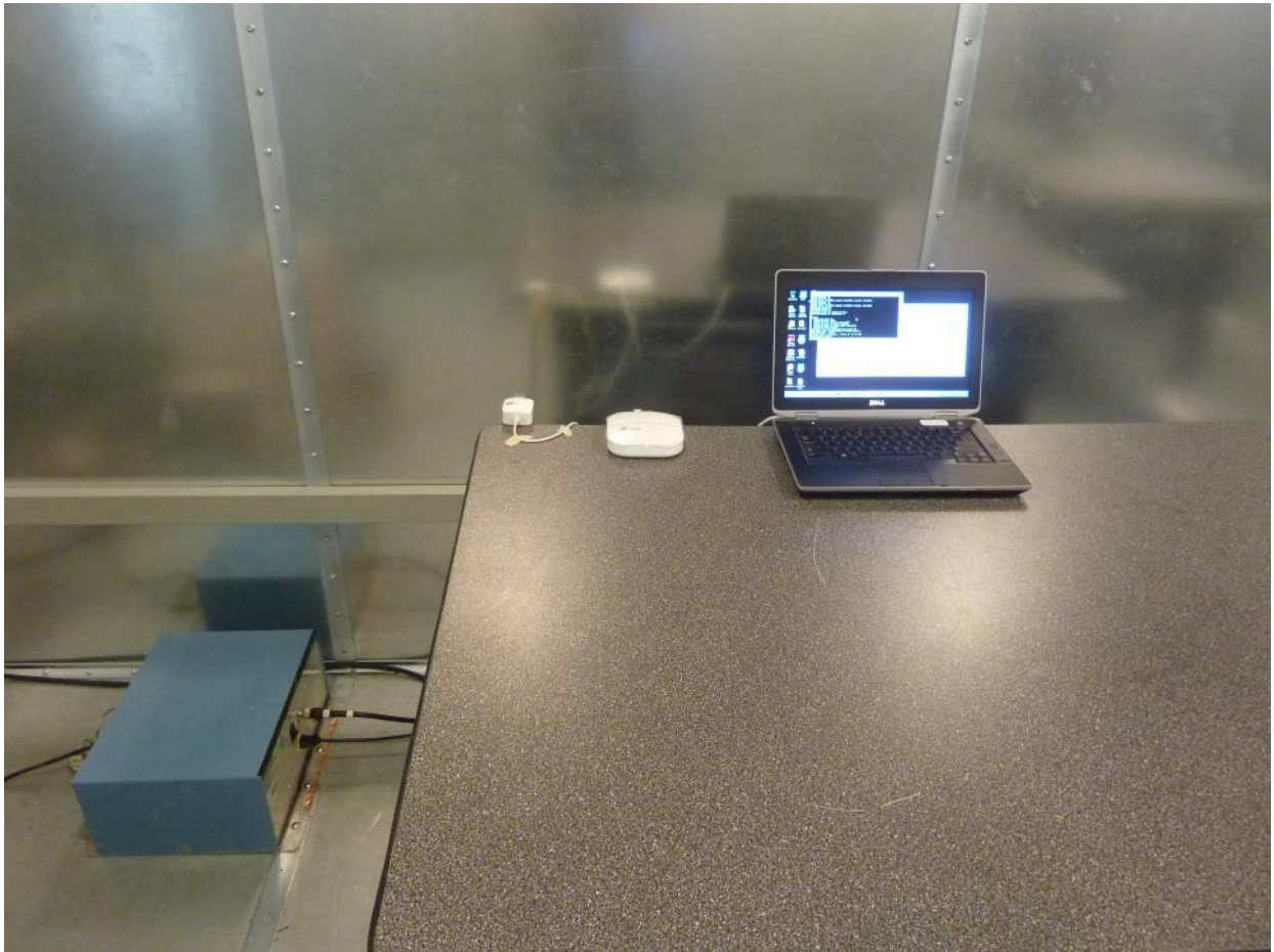
Figure 10: Conducted Emission Test Setup (Front)
