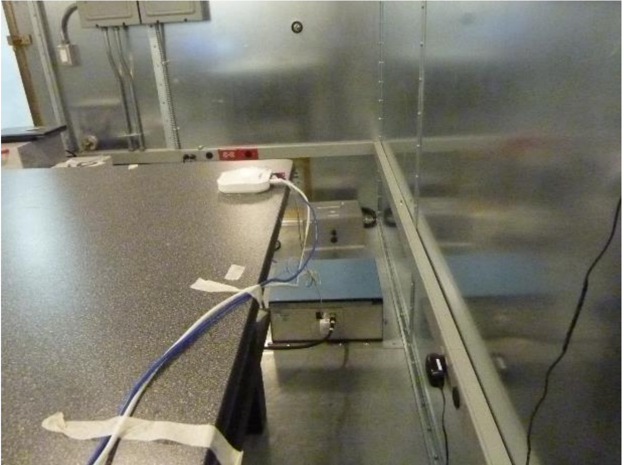
Figure 11: Conducted Emission Test Setup (Side)
