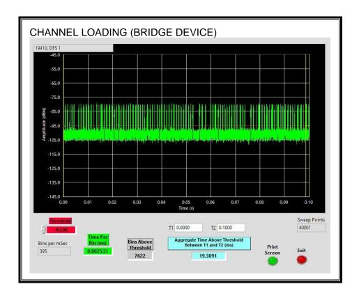
The level of traffic loading on the channel by the EUT is 19.30%
