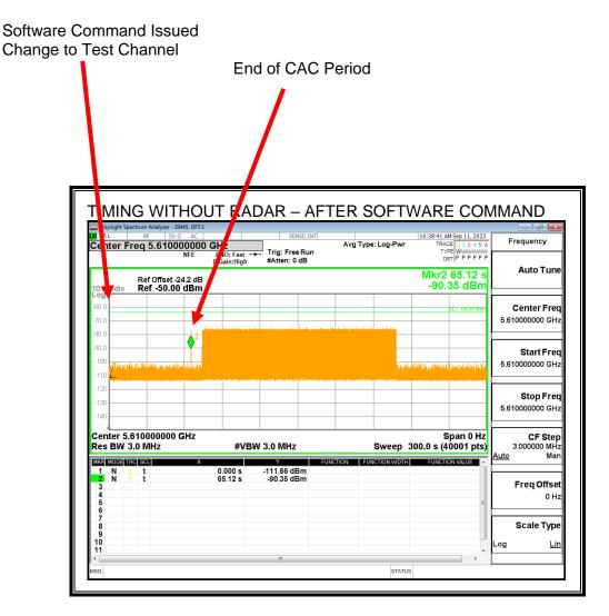
Transmissions begin on channel after completion of the initialization cycle and the CAC.
