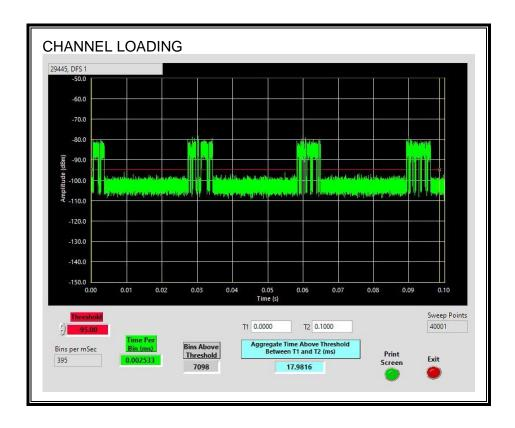
The level of traffic loading on the channel by the EUT is 17.98%
