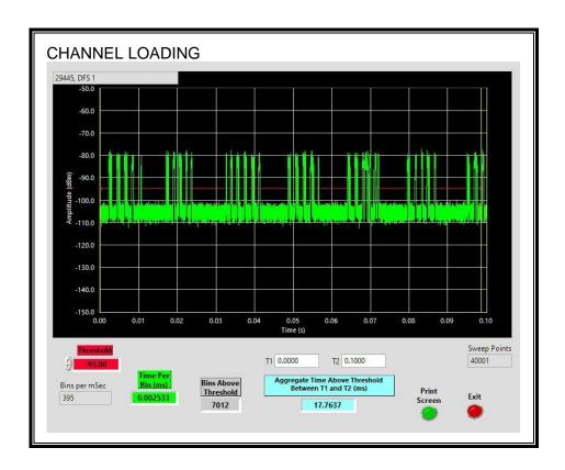
The level of traffic loading on the channel by the EUT is 17.76%
