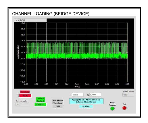
The level of traffic loading on the channel by the EUT is 19.79%
