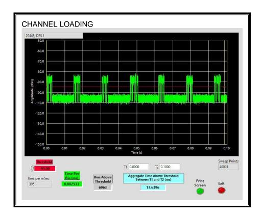
The level of traffic loading on the channel by the EUT is 17.64%
