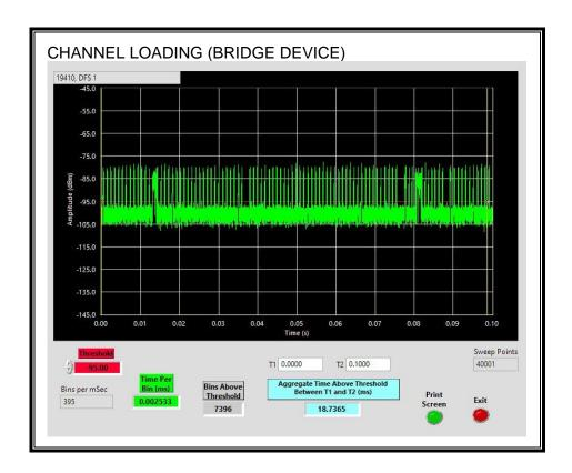
The level of traffic loading on the channel by the EUT is 18.73%
