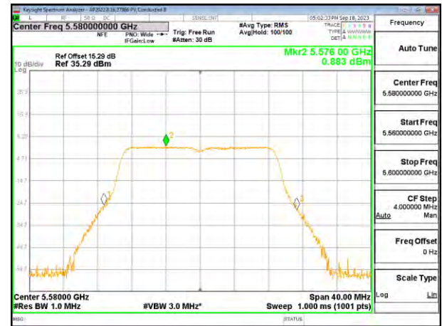
MID CHANNEL ANTENNA 4
