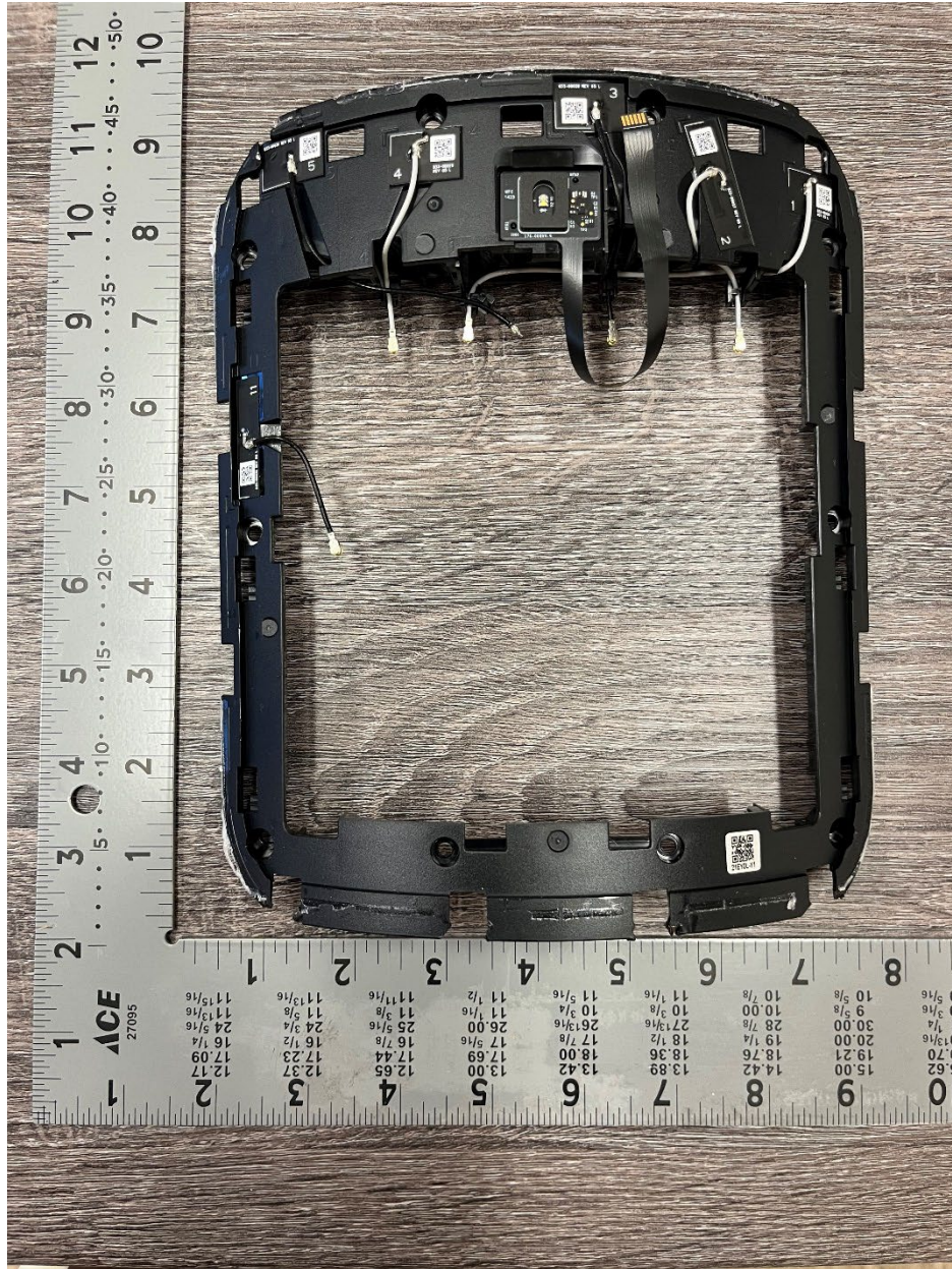
Figure 7. Antennas on antenna carrier; front side
