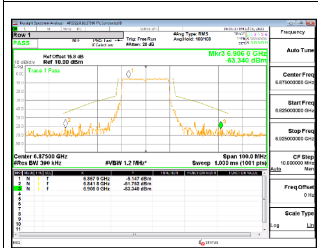
STRADDLE CHANNEL Antenna 3
