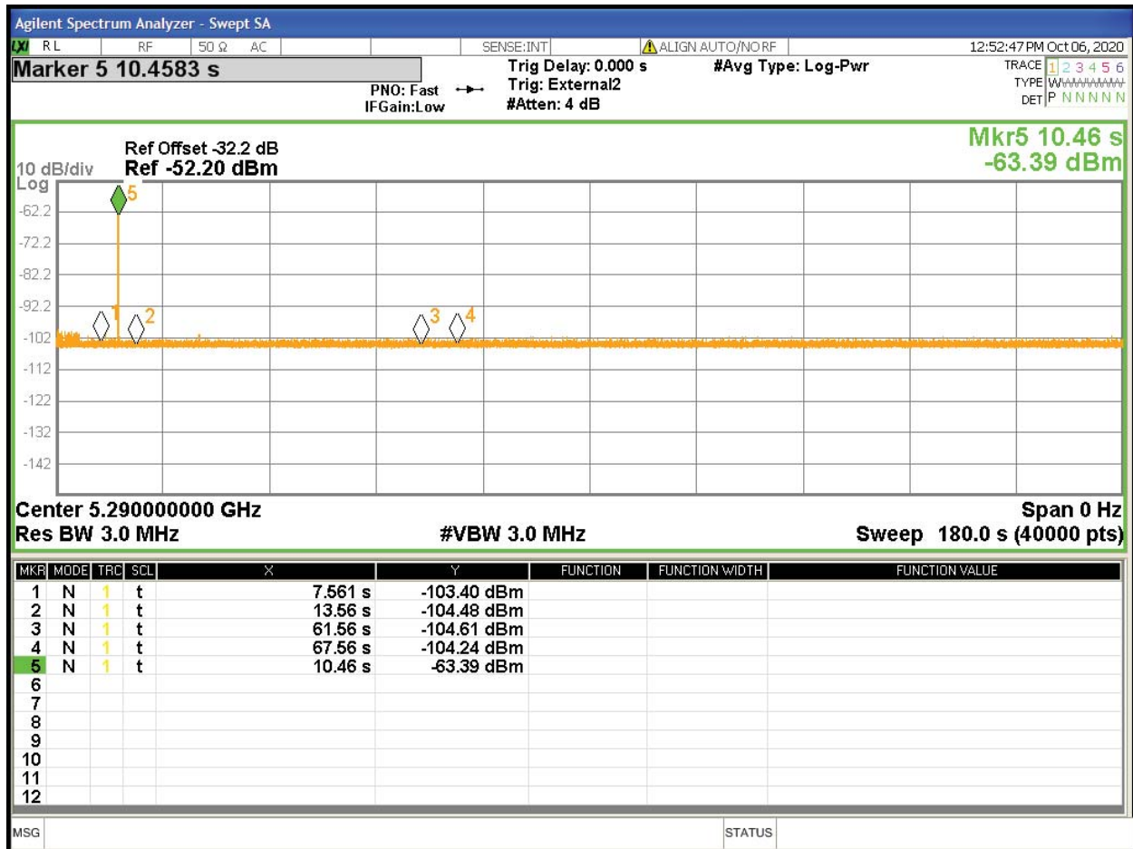
Figure 16: Radar Pulse Injection near the Beginning of Channel Availability Check for 80 MHz Bandwidth
