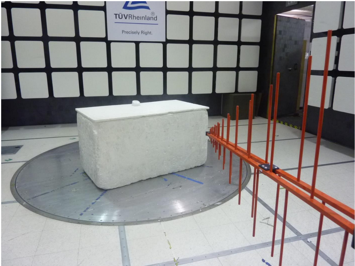
Figure 4: Test Setup for 30 MHz to 1 GHz (View 2)
