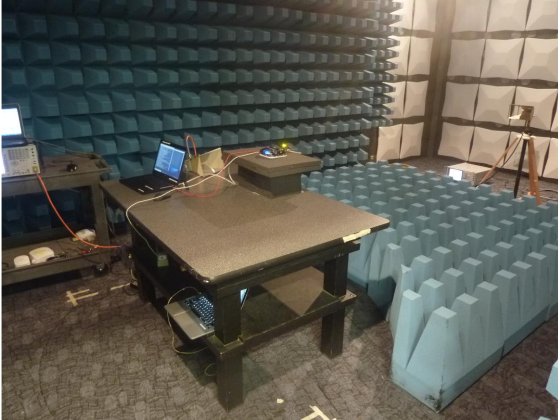
Figure 34: DFS Test Setup Photo for Master – Radiated Method – View 2
