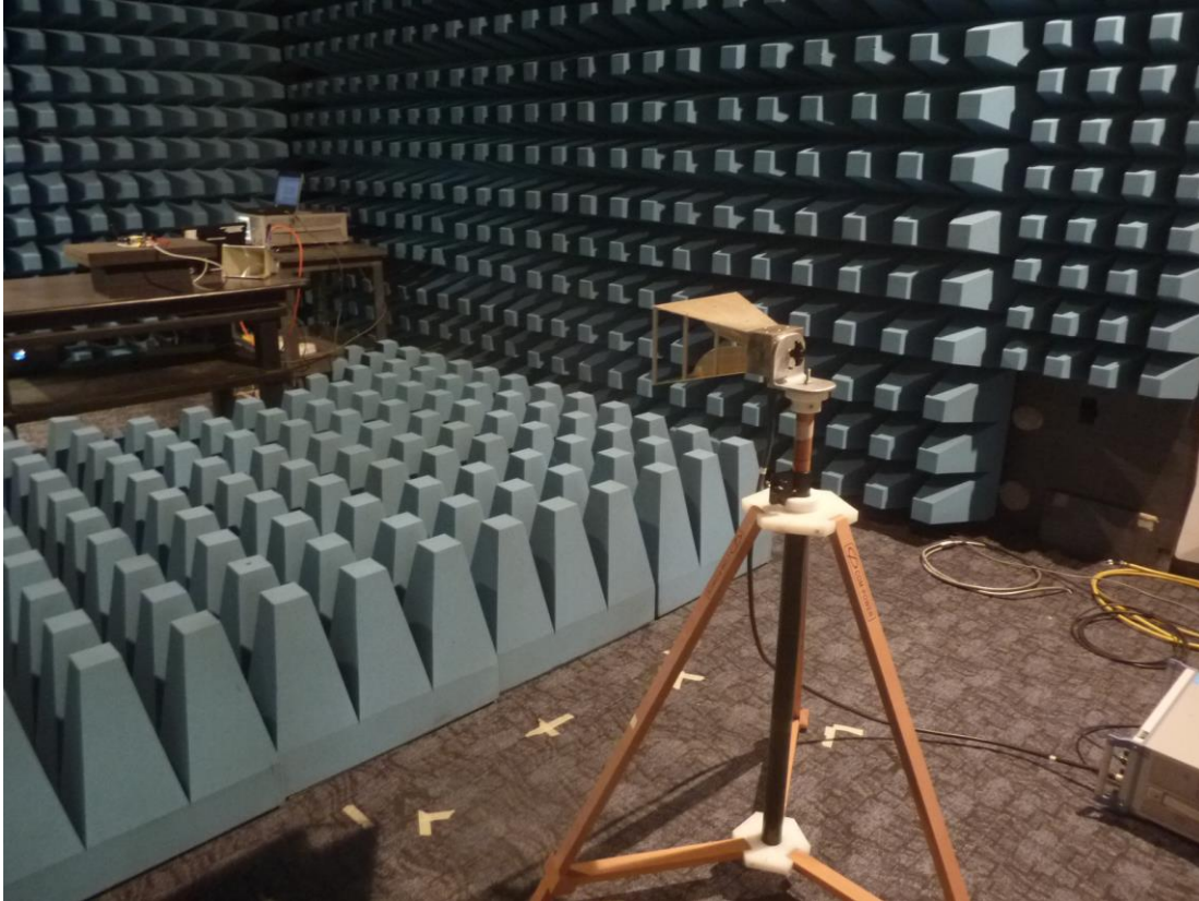
Figure 33: DFS Test Setup Photo for Master – Radiated Method – View 1
