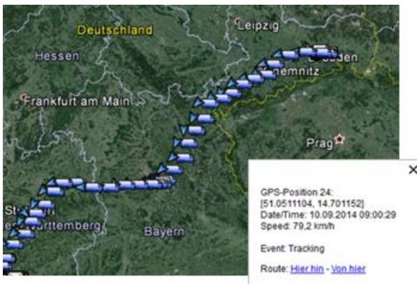
The up to 15,000 recorded position data sets, including speed and direction, can be imported afterwards into Google Earth or similar software and be evaluated.
