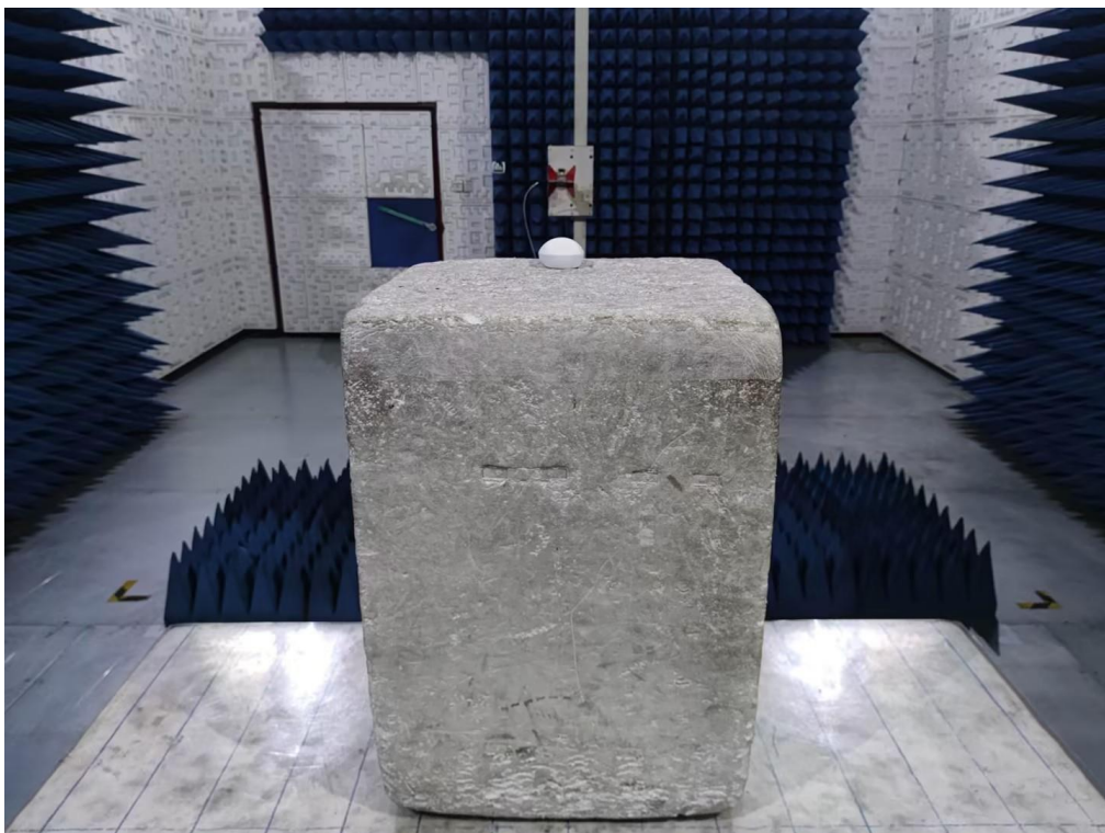
RADIATED EMISSION TEST SETUP ABOVE 1GHz
