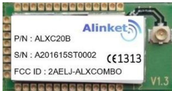
Figure 2 ALXC2X (External Antenna, U.FL Connector) Top View
