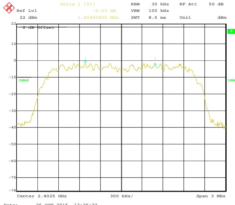
**EDR ( $\pi/4$ -DQPSK): Middle Channel**
