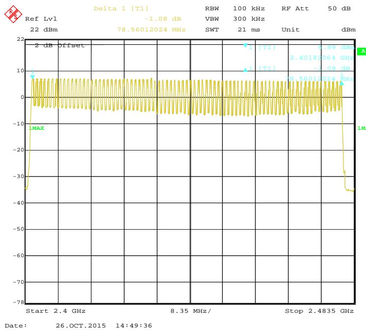
**EDR ( $\pi/4$ -DQPSK): Number of Hopping Channels**
