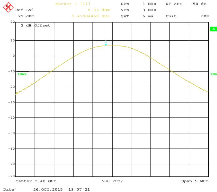
**EDR( $\pi/4$ -DQPSK): Low Channel**
