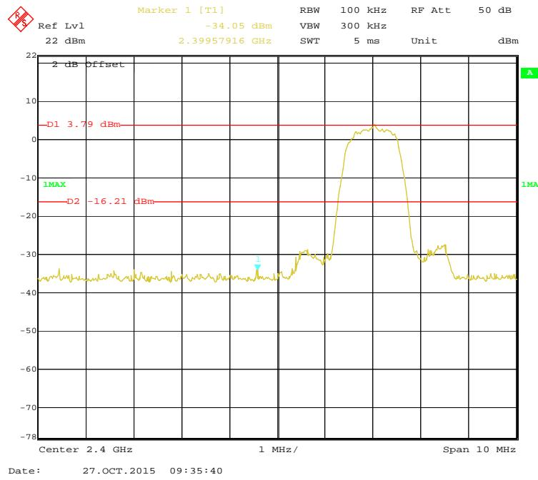
**EDR ( $\pi/4$ -DQPSK): Band Edge-Right Side**
