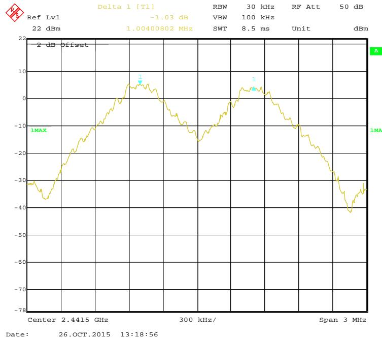
**BDR (GFSK): High Channel**
