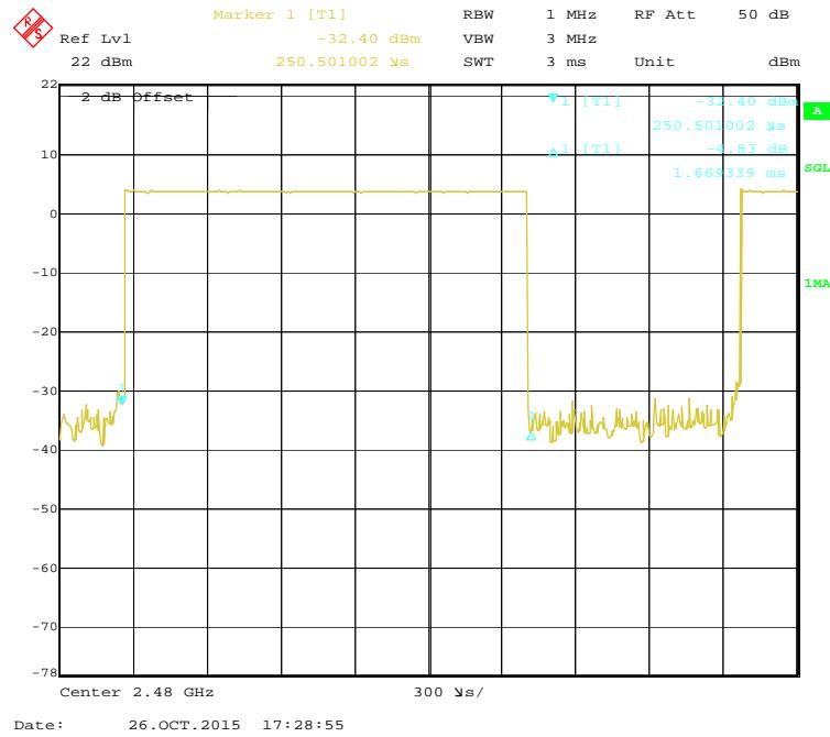
**Pulse time, Low Channel, DH5**
