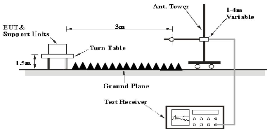
The radiated emission tests were performed in the 3 meters, using the setup accordance with the ANSI C63.10-2013. The specification used was the FCC 15.209 and FCC 15.247 limits.
