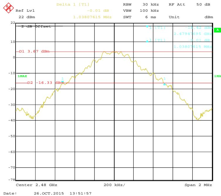
**EDR ( $\pi/4$ -DQPSK): Low Channel**
