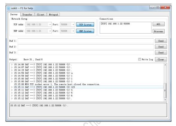
In the connected device list of the TCP server, select the IP address of the ALX82x Wi-Fi communication module, and send the "helloworld" string to the DAT:
