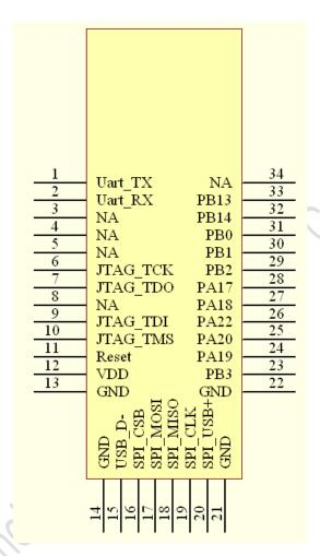
Notes: the pin mappings between IC and schematic are identical
