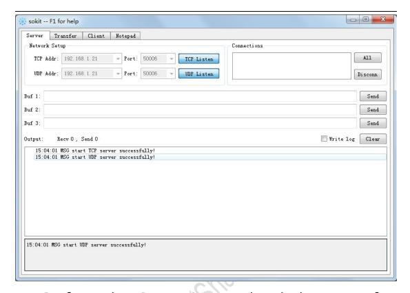
Configure the TCP/UDP Server, select the host IP interface which will be used to communicate with the ALX82x modules, and set the TCP/UDP port to 50006, then click "TCP/UDP Listen", with the same configuration the ALX82x modules should automatically connect to our TCP/UDP server:
