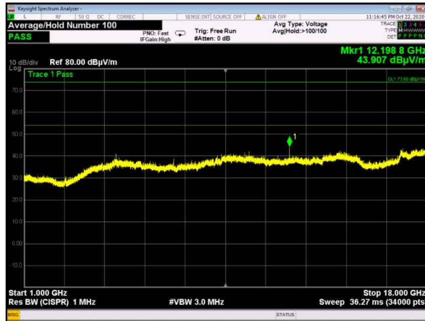
Plot 4.4.1.13: Radiated Spurious Emission in 1 – 18 GHz range, F_c = 2440 MHz, Vertical Polarization, Peak
