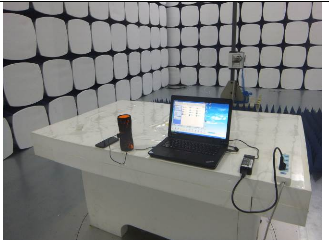
Radiated Spurious Emissions Test Setup Above 1GHz
