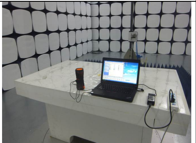
Radiated Spurious Emissions Test Setup Above 1GHz
